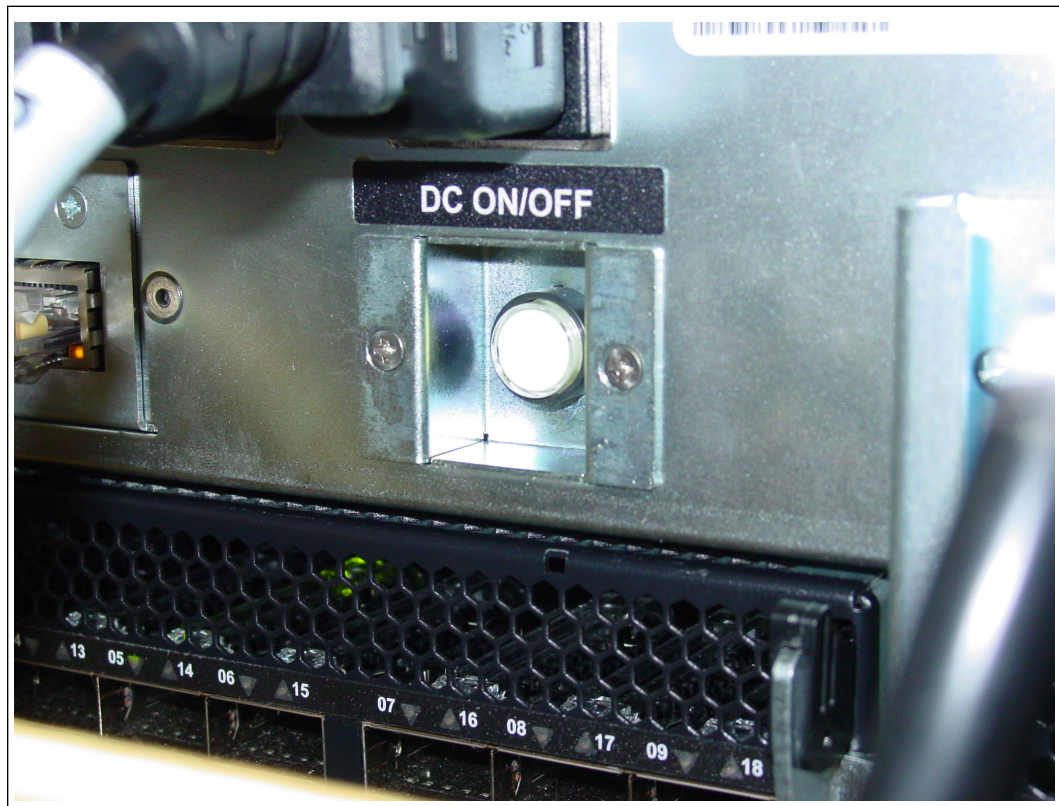
Figure 43. DC ON/OFF Switch
