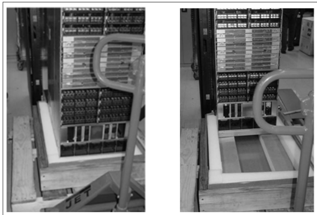
Figure 37. Sliding the Switch off the Pallet
