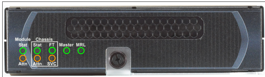
Figure 56. Management Module LEDs
