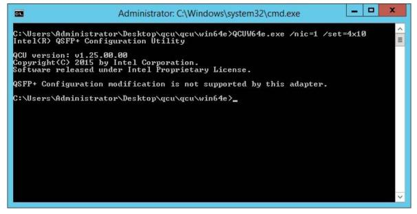
Figure 6. QSFP+ Configuration Modification Not Supported
