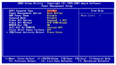
Figure 3-7A. Power Management Setup Main Menu
