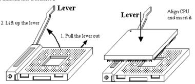
Figure 2-1. Socket A and open its lever
