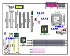
Attach the connector from the CPU fan to the header named FAN1 ond connector from the chassis fan to the header FAN2 (These two fan headers have a sense signal that can detect fan rotation speeds) or FAN4 and attach the connector from the power fan to FAN3 header. FAN5 is for the northbridge chipset fan.
