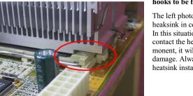
The left photo shows the bottom right side of the heaksink in contact with the right side of the Socket. In this situation, the processor die does not properly contact the heatsink. If you start the computer at this monent, it will immediately cause the processor damage. Always check this place when you finish the heatsink installation.
