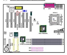
There is a specific orientation for pins 1 through 5, attach the connector from the IR KIT or IR device to the IR1 header. This motherboard supports standard IR transfer rates.
