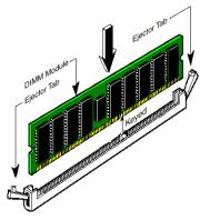
Figure 2-6. DDR DIMM module installation
