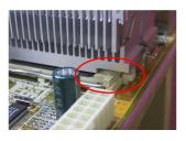
The left photo shows the bottom right side of the heaksink in contact with the right side of the Socket. In this situation, the processor die does not properly contact the heatsink. If you start the computer at this monent, it will immediately cause processor damage. Always check this location when you finish the heatsink installation.
