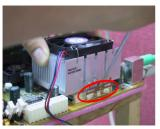
Check the photo on the left. You have finished the heatsink installation. Now hold the whole heatsink and slightly shake it, make sure the bottom right side of the heaksink does not contact the right side of the Socket (see bottom picture). Otherwise, the processor die does not have proper contact with the heatsink. This situation
