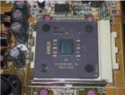
First, install the processor into the processor socket.
