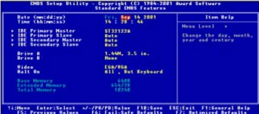
Figure 3-3A. Standard CMOS Setup Screen Shot
