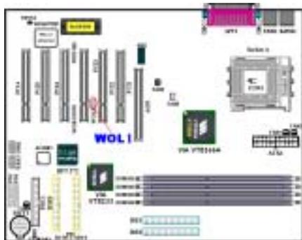
If you have a network adapter that supports this feature, then you can connect the specific cable from the network adapter to this header. This feature lets you wake up your computer via remote control through a local area network. You may need a specific utility to control the wake up event, like using the PCnet Magic Packet utility or other similar utilities.
