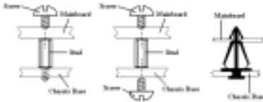
Figure 2-2. The way we fixed the motherboard
