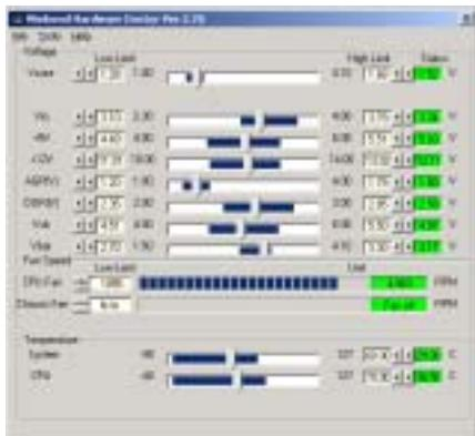
This screen shows the hardware monitor system screen. It shows information about system temperature, voltages and fan speed. Some items can let you set the warning range; you can optimize values by setting them in accordance your system.
