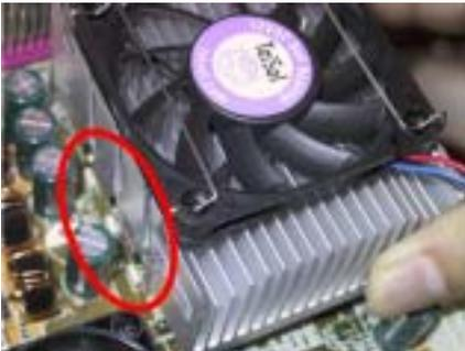
Insert the heatsink left side fix plate into the processor socket left side fix hooks. Make sure the fit is very tight. Check the photo on the left.
