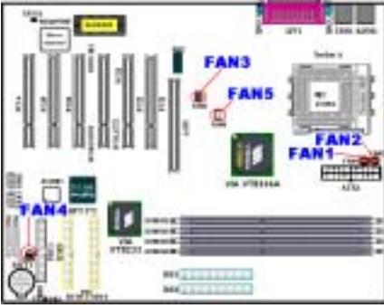
Attach the connector from the CPU fan to the header named FAN1 and connector from the chassis fan to the header FAN2 (These two fan headers have a sense signal that can detect fan rotation speeds) or FAN4 and attach the connector from the power fan to FAN3 header. FAN5 is for the northbridge chipset fan.
