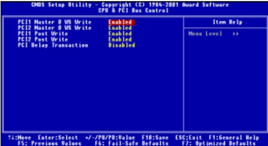
Figure 3-5D. CPU & PCI Bus Control Screen
