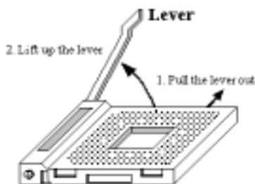
Figure 2-3. Socket A and open its lever
