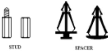
Figure 2-1. The outline of stud and spacer
