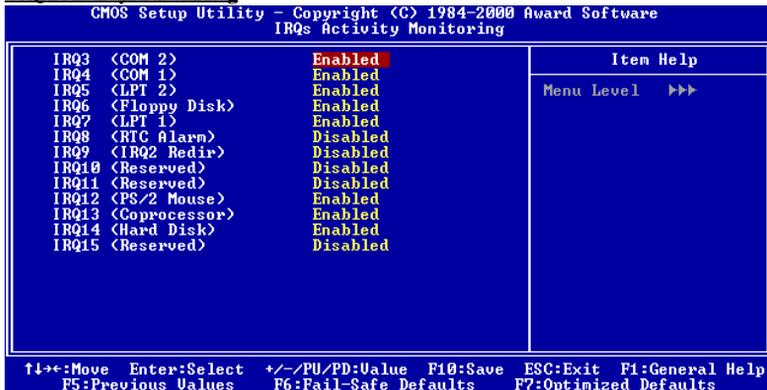
Figure 3-7D. Menu de l'IRQs Activity Monitoring Setup
