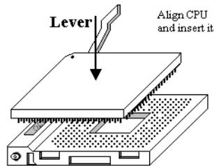
Figure 2-4. Install the CPU into socket A
