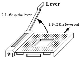
Figure 2-3. Socket A and open its lever
