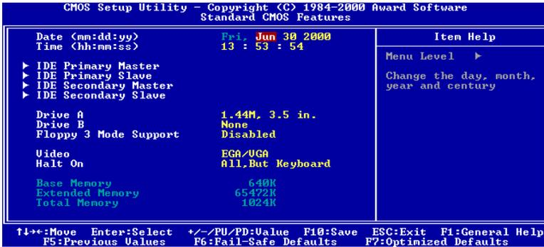
Figure 3-3A. Ecran du Standard CMOS Setup
