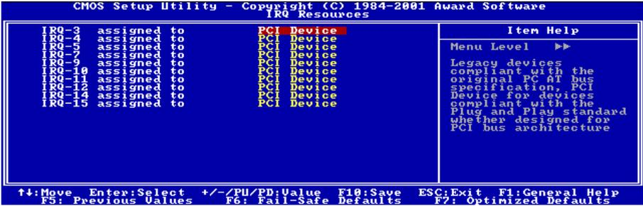
Figure 3-9. PnP/PCI Configurations – Menu IRQ Resources
