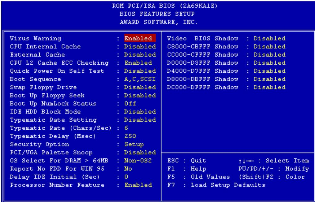
Fig 3-4 BIOS Features Setup
