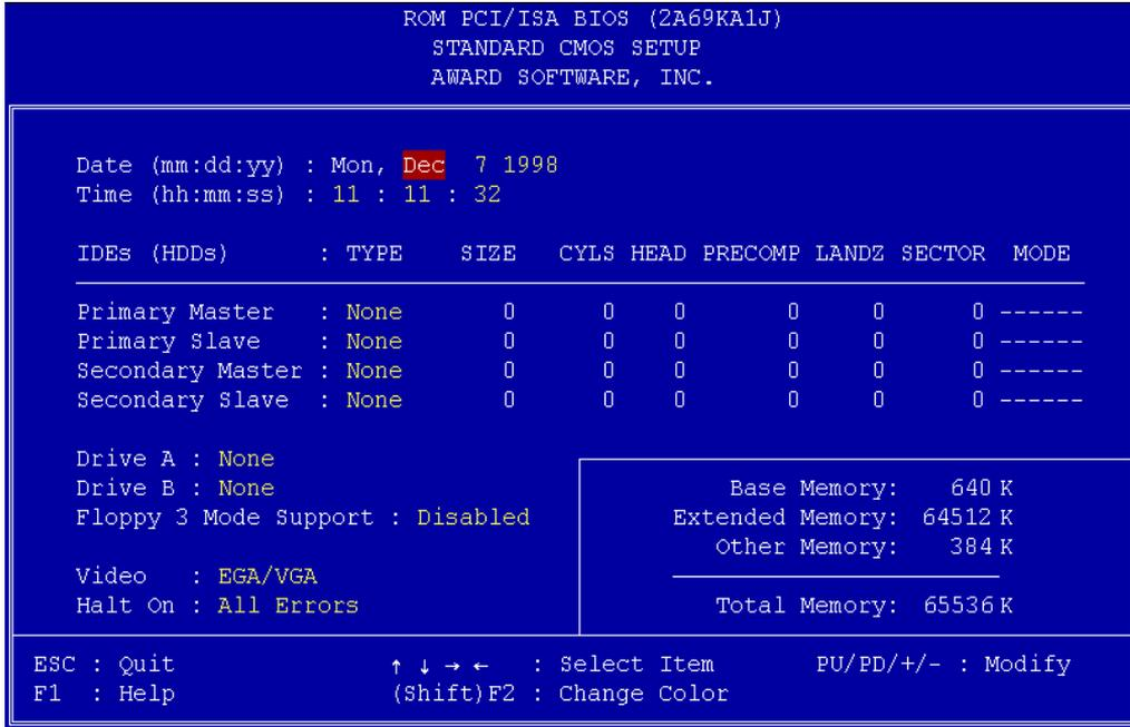
**Fig 3-3 Standard CMOS Setup Menu**
