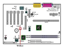
If you have a Network adapter that supports this feature, then you can connect the specific cable from the network adapter to this header. This feature lets you wake up your computer via remote control through a local area network. You may need a specific utility to control the wake up event, like using the Intel<sup>®</sup> LDCM<sup>®</sup> utility or other similar utilities.
