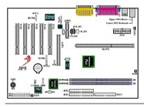
This jumper lets you select the CODEC mode on the AMR card. When pin 1 and pin 2 jumpers are shorted (default), the CODEC on the AMR card is set to secondary mode. If pin 2 and pin 3 jumpers are shorted, the onboard audio CODEC is disabled and CODEC on the AMR card is set to primary mode.
