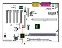
The RT2 is for you to connect an additional thermistor to detect the temperature in the location of your choice. You can buy the thermistor at an electronics store, and ask for a  $10K\Omega$  thermistor which should be OK. Please don't use too long of a lead wire for the thermistor.
