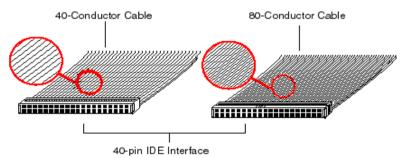
Figure 2-9. The difference between Ultra ATA/33 and Ultra ATA/66 Conductor Cables
