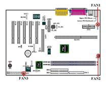
FAN1, FAN2 & FAN3: FAN header
