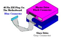
Figure 2-11. How to connect an ATA/66 Cable to the Motherboard
