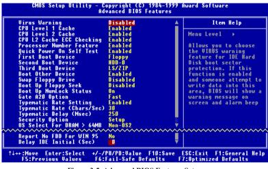
Figure 3-5. Advanced BIOS Features Setup
