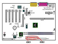
An IDE hard disk drive ribbon cable has 40 wires and two connectors to provide a connection for two IDE hard disk drives. After connecting the single end to the IDE1 (or IDE2), connect the two connectors on the other end to the IDE hard disk drives (or CD-ROM drive, LS-120, etc.).
