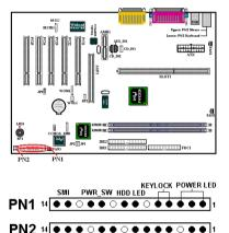
PN1 and PN2 are for switches and indicators for the chassis's front panel, there are several functions that come from these two headers. You have to watch the pin position and the orientation, or you may cause system malfunctions. Figure 2-8 shows you the PN1 and PN2 functions of the pins.
