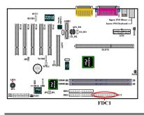
This 34-pin connector is called the "*floppy disk drive connector*". You can connect a 360K, 5.25", 1.2M, 5.25", 720K, 3.5", 1.44M, 3.5" or 2.88M, 3.5" floppy disk drive, you can even connect a 3 Mode floppy disk drive (it's a 3 1/2" drive used in Japanese computer systems).
