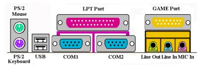
Figure 2-12. CX6 back panel connectors
