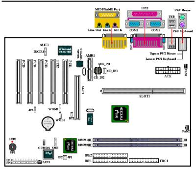
Figure 1-1. Motherboard component location
