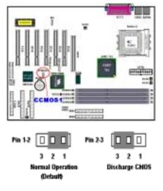
Jumper CCMOS1 discharge CMOS memory. When you install the motherboard, make sure this jumper is set for normal operation (pin 1 and 2 shorted). See Figure 2-8.
