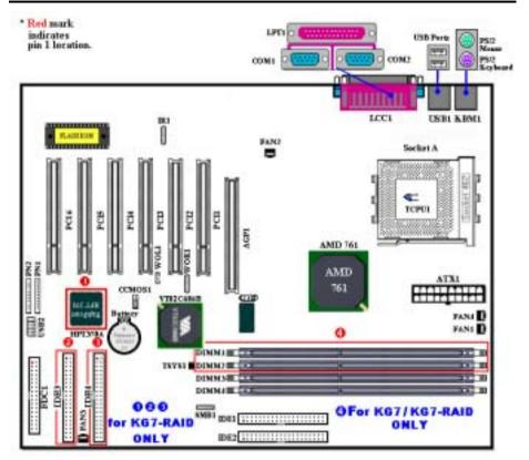
Figure 1-1. KG7-Lite/KG7/KG7-RAID motherboard component location
