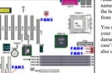
Attach the connector from the CPU fan to the header named FAN4 ond connector from the chassis fan to the header FAN1 or FAN3 and attach the connector from the power fan to FAN2 header.
