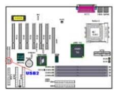
This header is for connecting the additional USB port plugs. You can use the special USB port expansion cable (optional). It provides two additional USB plugs. These USB plugs can be fixed on the back panel.
