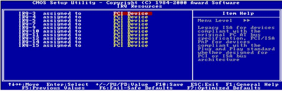
Figure 3-10. PnP/PCI Configurations – Menu IRQ Resources
