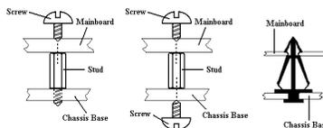
Figure 2-2. The way we fixed the motherboard
