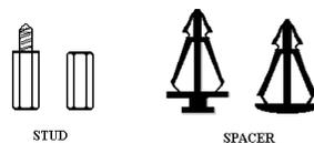
Figure 2-1. The outline of stub and spacer
