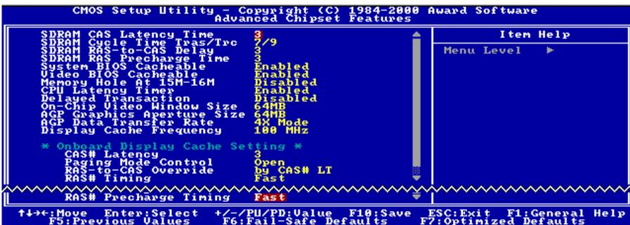
Abb. 3-6 Advanced Chipset Features Setup
