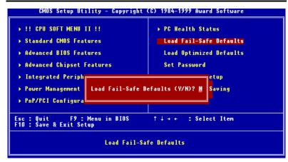
Figure 3-12. Load Fail-Safe Defaults
