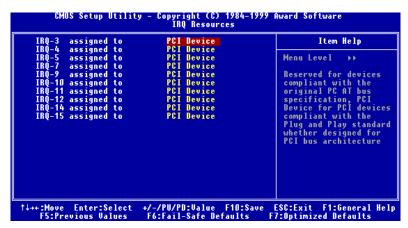
Figure 3-10. PnP/PCI Configurations - Menu IRQ Resources
