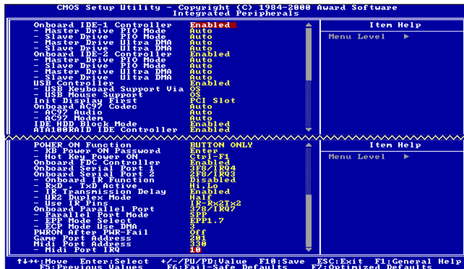
Figure 3-7. Menu de l'Integrated Peripherals
