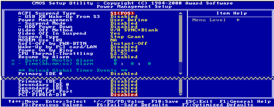
Figure 3-8. Menu de l'Power Management Setup
