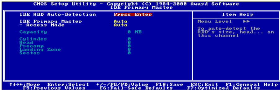
Abb. 3-4. IDE Primary Master Setup
